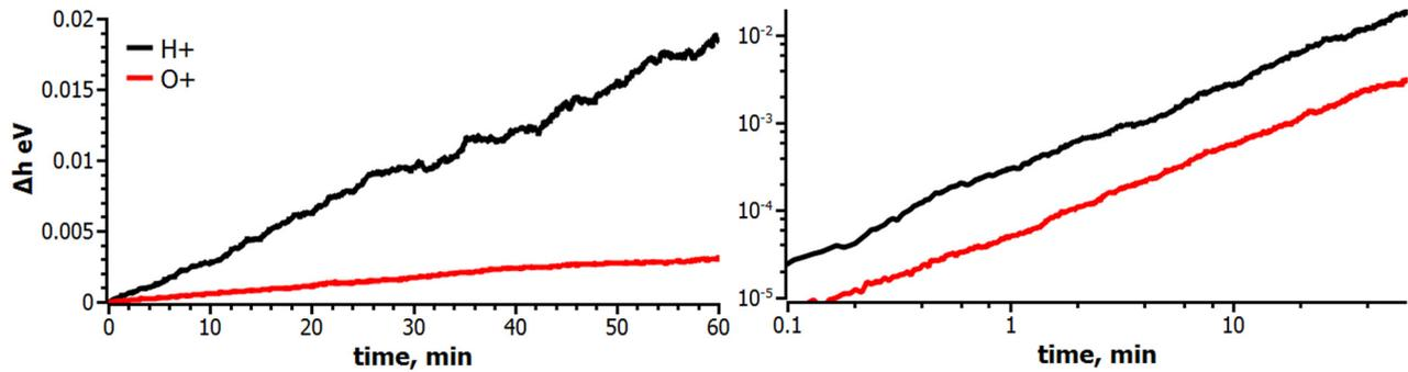
FIG. 5. Transverse ion heating by random EMIC wave packets at  $L=2.5$ , using realistic time-averaged root-mean-squared EMIC wave amplitude  $E=0.015$  mV/m,  $f=0.03a \sin(\tau/a)$ ,  $a=60/\pi$ , and  $b=3$  in Equation (5), corresponding to EMIC frequency  $f \sim 12$  Hz,  $\tau_c \sim 0.2$  s, and  $T_{cp} = 1/28$  s. Black and red curves show  $H^+$  and  $O^+$  ion heating, respectively, as a function of time (left and right panels show linear and logarithmic scales).
