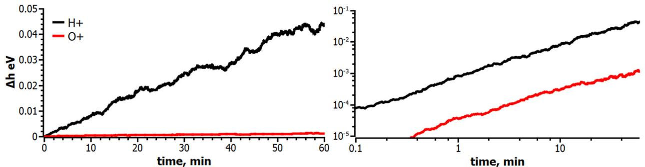
FIG. 4. Transverse ion heating by random hiss wave packets at  $L = 2.5$ , using realistic time-averaged root-mean-squared hiss amplitude  $E = 0.05$  mV/m,  $f = a \sin(\tau/a)$ ,  $a = 2.5/\pi$ , and  $b = 5$  in Equation (5), corresponding to hiss frequency  $f \sim 350$  Hz,  $\tau_c \sim 0.014$  s, and  $T_{cp} = 1/28$  s. Black and red curves show proton and  $O^+$  ion heating, respectively, as a function of time (left and right panels show linear and logarithmic scales).
