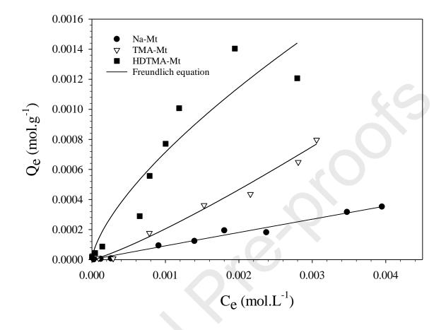
**Fig. 4.** Adsorption isotherms at the equilibrium of the batch adsorption experiments of the AMX onto Na-Mt, TMA-Mt and HDTMA-Mt and their fitting with the use of a Freundlich model.
