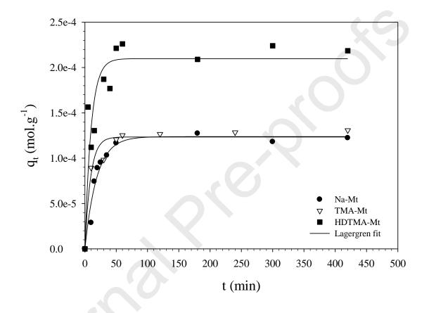
**Fig. 5.** Kinetics adsorption isotherms of the batch adsorption experiments of the AMX onto Na-Mt, TMA-Mt and HDTMA-Mt and their fitting with the use of a pseudo-first order model.
