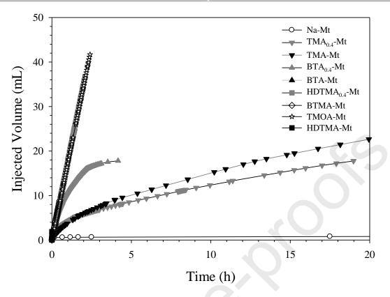
**Fig. 2.** Representation of the injected volume of water as a function of the time (in h) for the characterization of the hydric behavior of the whole organoclays as well as the raw clay mineral.
