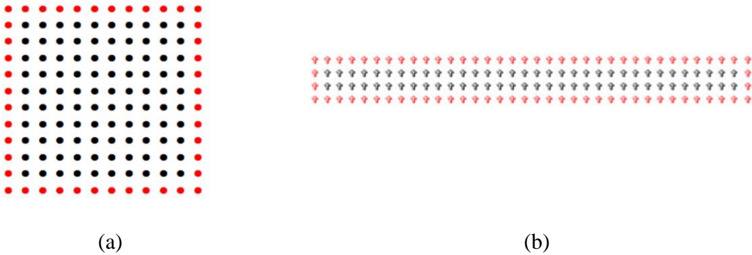
Figure 8. (a) Square lattice with size 12x12 with a number core atoms N_C = 100 and atoms at the edge, N_e = 44 . (b) Rectangle-shaped lattice with size 4x36, containing N_C = 68 core atoms and N_e = 76 edge sites. Black and red dots represent respectively the core ( N_C ) and the edge ( N_e ) lattice sites.
