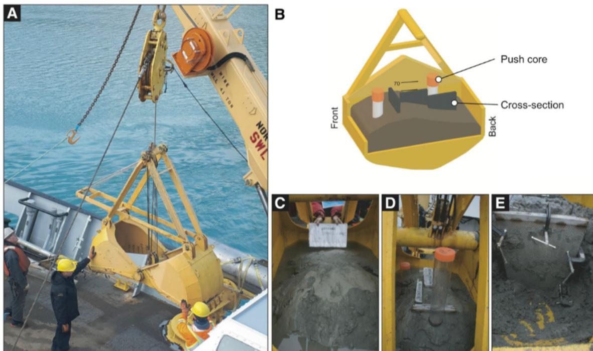
**Fig. 4.** Grab sampling. **(A)** IKU grab sampler ready for deployment. **(B)** 3D representation of an IKU grab with sediment inside. Cross sections and push cores were collected from the grab. **(C) to (E)** Examples of cross-sections being collected from the grab sampler.
