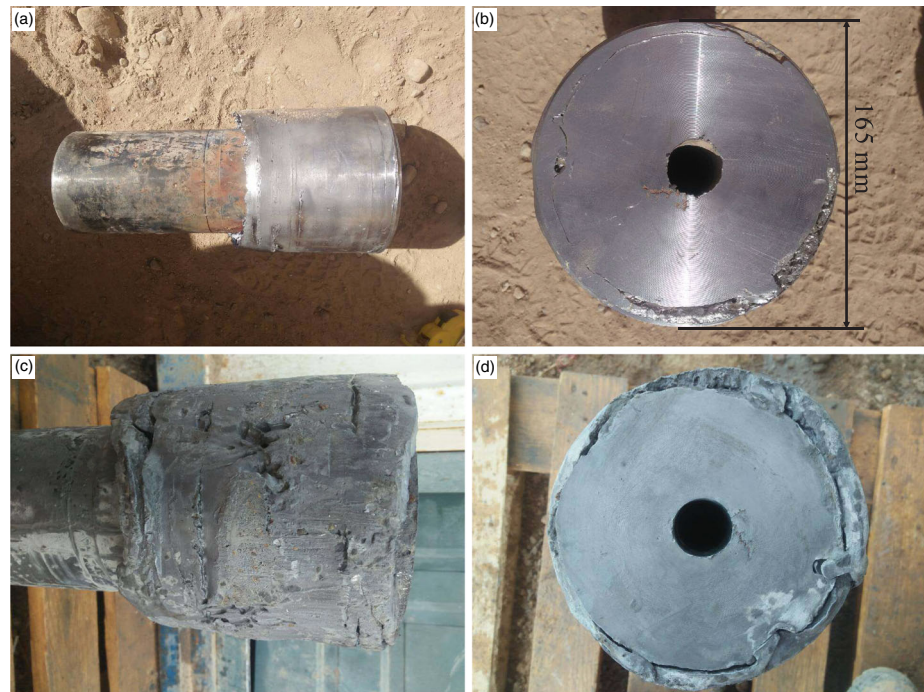
Figure 4. Photos of the lead seal before being put into (a and b) and after being pulled out (c and d) from borehole H4-3-414. The diameter of the lead seal bottom is 165 mm and the inner diameter of the casing pipe is 166.63 mm. The side face of the lead seal has scratches, but no imprint exists in its bottom surface, revealing that the coseismic slip at this borehole site is more than 196.85 mm, the outer diameter of the casing pipe.
