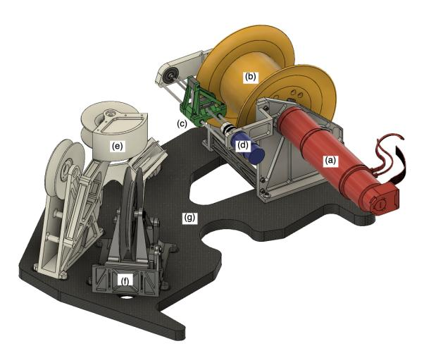
Figure 2: Rendering of RACHuTS reel system. Major assemblies include the primary drivetrain (a/red), reel (b/yellow), level wind carriage (c/green), level wind motor (d/blue), line redirection pulley train (e/white), kinematic pulley (f/grey) and carbon fiber baseplate (g/black twill), line, electronics box and docking connector are not shown.
