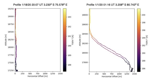
Figure 5: Horizontal offset of the profiling unit relative to the Zephyr gondola, color coded by ambient temperature. (a) A low wind shear example demonstrating < 100m horizontal displacement and a nearly isothermal profile. (b) High wind shear example with 1400m horizontal displacement and 14K temperature gradient. The difference in motor torque between these profiles is 4.7%.
