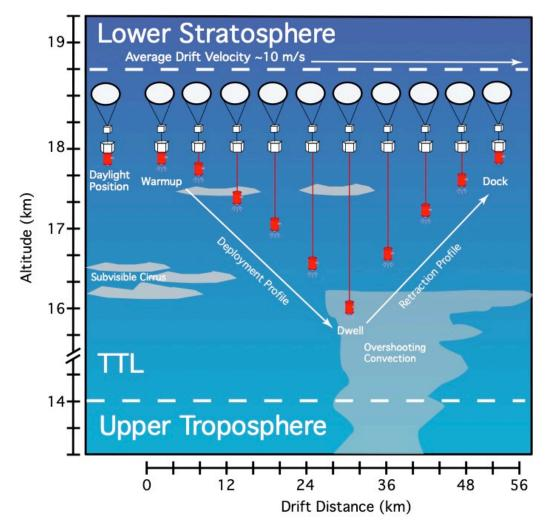
Figure 1: RACHuTS Operational Concept. The RACHuTS Profiler is deployed from a super pressure balloon at 18.5km, down to an altitude of 16.5km 3-5 times per night making measurements of water vapor, aerosol, cloud particles, temperature and pressure.
