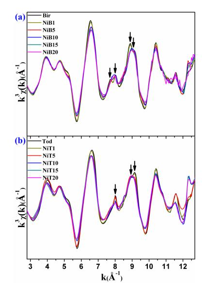
Fig. 8. Mn K-edge EXAFS spectra obtained for (a) layered precursors and (b) reflux
