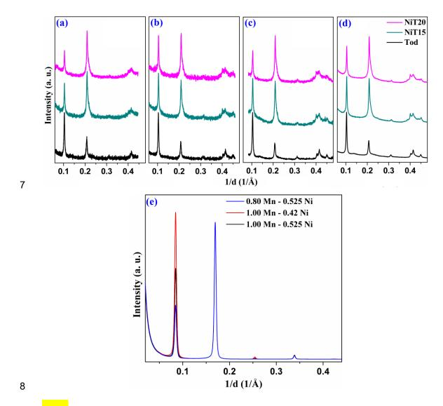
Fig. 2. XRD patterns collected for NiT20, NiT15, and Tod at (a) Mn K-edge (6.5 keV),
