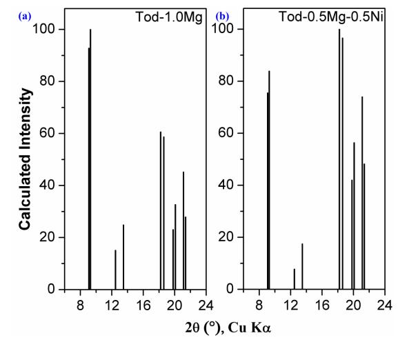
Fig. 12. Intensity distributions calculated for ideal todorokite (ICDD #38-0475) with (a) only Mg in todorokite tunnels and (b) with Mg and Ni present in a 1:1 ratio in todorokite tunnels. In both cases, the model of Post et al.(2003) was modified assuming the complete filling of the O8 site by  $H_2O$  molecules (no cations) and the presence of 1.0 cation (Mg or Mg+Ni) in the Mg site.
