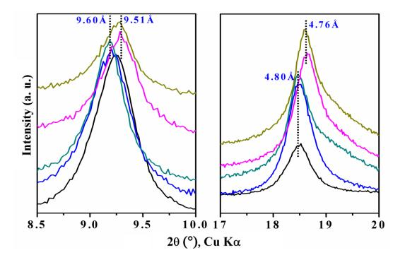
Fig. S2. XRD patterns of reflux products (zoom on low-angle regions). Colors as in Fig. 1.
