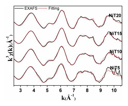
Fig. S5. Linear combination fitting of NiT K-edge EXAFS spectra using Ni(OH)<sub>2</sub> and corresponding NiB samples as standard references.
