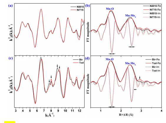
Fig. 9. Comparison of (a, c) Mn K-edge EXAFS and (b, d) of their FTs (showing both
