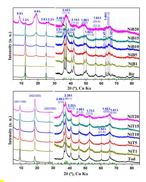
Fig. 1. XRD patterns of layered precursors (top) and reflux products (bottom). Colors
