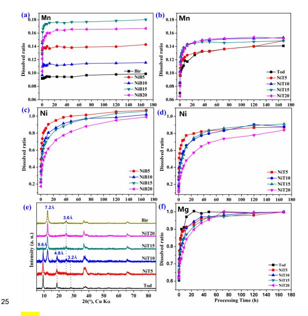
Fig. 5. Proportion of metal cations released during the nitric acid treatment: (a-b): Mn, (c-d): Ni, and (f): Mg. The amount of metal released is normalized to the sample overall metal content (see text for details). (e): XRD patterns of samples treated with nitric acid. Colors as in Fig. 1 except for Bir in (e).
