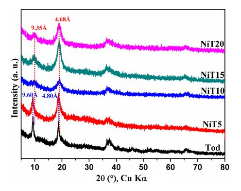
Fig. S3. XRD patterns of reflux products after heating to 140 °C for 12 hours. Colors as in Fig. 1.
