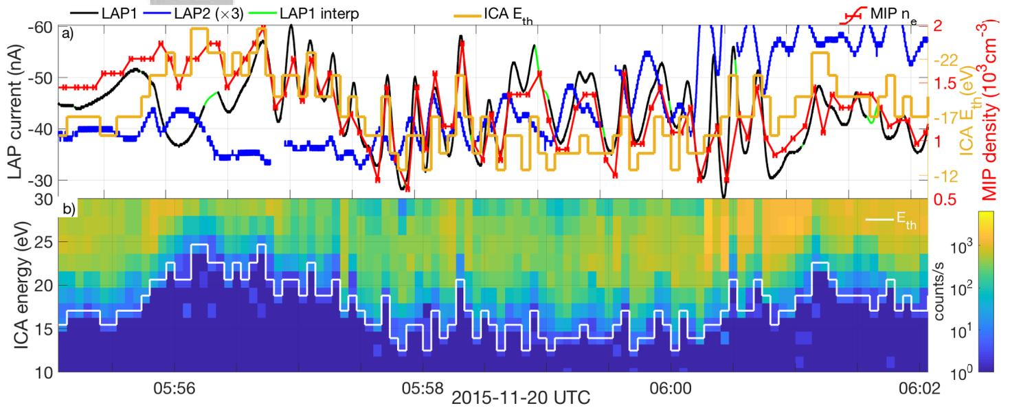
**Figure 3.** Multi-instrument wave observations on 20 Nov 2015. a) LAP1 & 2 probe currents (black and blue lines, respectively, to be read off the left-hand y-axis, green segments indicate data gap interpolation, see section A.1), MIP density and ICA spacecraft potential estimates (red and yellow lines, to be read off the correspondingly coloured right-hand y-axes) b) ICA ion energy spectra with the lower edge  $E_{th}$  identified as described in the text.
