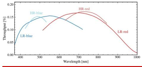
**Figure A1** - MAVIS spectrograph throughput in each of the four spectral modes. Throughput includes telescope, AOM, spectrograph optics, and detector quantum efficiency.
