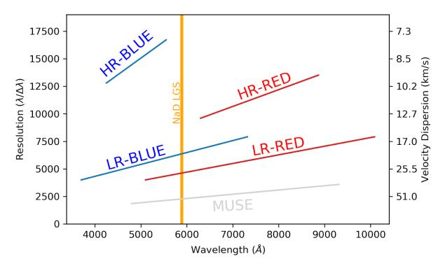
*Figure 6.5:* Summary of MAVIS spectral modes, showing wavelength coverage and spectral resolution. Left axis indicates resolution, computed as wavelength/FWHM. Right axis shows these values in terms of velocity dispersion, indicating the minimum line widths that can be securely measured. MUSE is overplotted for comparison.
