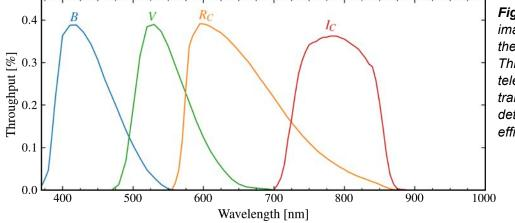
**Figure A2** - MAVIS imager throughput in the VBR<sub>c</sub>I<sub>c</sub> filters. Throughput includes telescope, AOM, filter transmission, and detector quantum efficiency.
