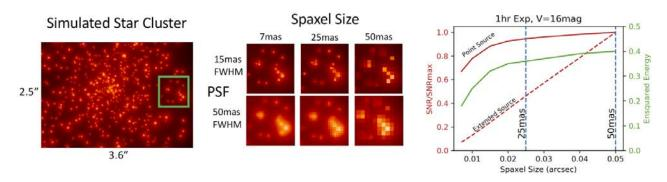
*Figure 6.6:* Left - Simulated star cluster in the MAVIS IFU field of view. Green box shows the field used in the middle thumbnails illustrating the Fine and Coarse IFU spaxel sizes for two different PSF extremes. Right - Growth curves of S/N and ensquared energy with spaxel size for a typical MAVIS source brightness.
