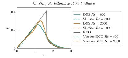
FIGURE 8. Mean azimuthal velocity in the DNS and semi-linear models at t = 60 for Ro = -4 for Re = 800 and Re = 2000. KCO indicates the velocity distribution predicted by Kloosterziel *et al.* (2007) in the inviscid limit. Viscous-KCO corresponds to the velocity profile (5.11) which takes into account viscous effects.
