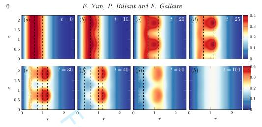
FIGURE 2. Vertical cross-sections at x = 0 of the evolution of the azimuthal velocity field v in DNS for  $k_m = 5.6$ , Ro = -4, Re = 800. The dashed lines delimit the regions where  $\phi < 0$  based on the mean azimuthal velocity  $\bar{v}$ . Only two wavelengths are shown whereas the full domain contains 13 wavelengths along the vertical (see §3.3).
