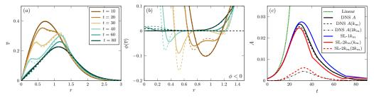
FIGURE 3. (a) Mean azimuthal velocity  $\bar{v}$  from DNS (solid lines) and SL-1 $k_m$  model (dashed lines), (b) corresponding Rayleigh discriminant  $\bar{\phi}$  and (c) perturbation amplitudes A as a function of time for Ro = -4 and Re = 800.
