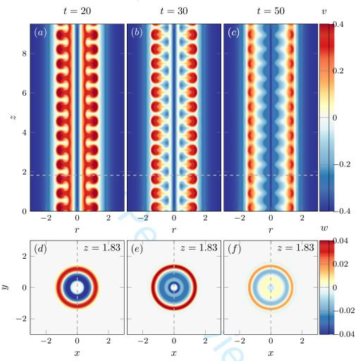
FIGURE 4. Evolution of the azimuthal velocity (a, b, c) and axial velocity (d, e, f) in a DNS for  $k_m = 8.6$ , Ro = -4, Re = 2000. (a, d) t = 20, (b, e) t = 30 and (c, f) t = 50. The vertical cross-sections (a, b, c) are at x = 0 and the horizontal cross-sections (d, e, f) at z = 1.83. The location of the different cross-sections are indicated by the dashed lines.
