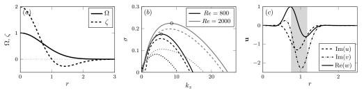
FIGURE 1. (a) Angular velocity  $(\Omega)$  and axial vorticity  $(\zeta)$  of the base flow. (b) Linear growth rate as a function of the vertical wavenumber k for different azimuthal wavenumbers: m = 0(solid lines), m = 1(dashed lines), m = 2(dotted lines) for Re = 800(black lines) and Re = 2000(grey lines) for Ro = -4 The circles indicate the most unstable modes. (c) Most unstable eigenmode for Re = 800. The shaded area indicates the region where  $\phi < 0$ .
