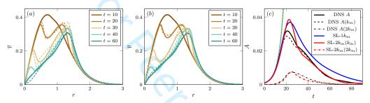
FIGURE 6. (a) Mean azimuthal velocity from DNS (solid lines) and semi-linear model  $\text{SL-}1k_m$  (dashed lines) and (b) for  $\text{SL-}2k_m$  (dashed lines). (c) The perturbation amplitudes A as a function of time for Ro = -4 and Re = 2000 for both  $\text{SL-}1k_m$  and  $\text{SL-}2k_m$ .
