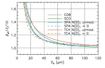
**Figure 12.**  $\beta_{\text{eff}} 12/10$  vs.  $D_{\text{e}}$  for the V4 LUTs (purple: CO8; green: SCO) and as derived by Mitchell et al. (2018) during the SPARTI-CUS (blue) and TC4 (red) field experiments using  $N(D)_1$  unmodified (solid) or  $N(D)_1 = 0$  (dashed).
