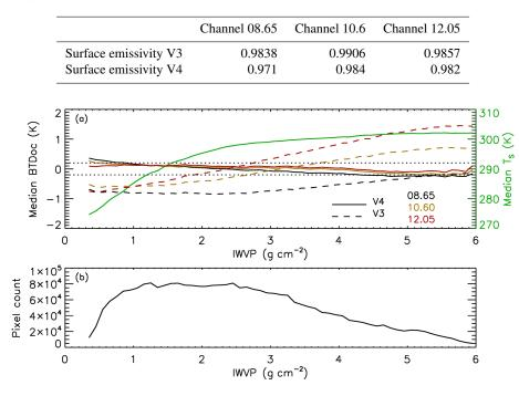
Table 1. Surface emissivity over oceans in the three IIR channels in V3 and in V4.
