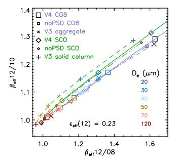
**Figure 11.** The V4 ice LUT values (solid lines; CO8: large squares; SCO: large diamonds) are compared with the V4 LUT values with no PSD (dashed–dotted lines and small symbols) and the V3 ice LUT values (dashed lines; cross: aggregate; plus signs: solid column) for six values of  $D_e$  between 20 and 120 µm and using  $\varepsilon_{eff,12} = 0.23$  for the three configurations.
