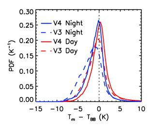
**Figure 8.** Probability density functions of the V4 (solid) and V3 (dashed) nighttime (blue) and daytime (red) differences between measured brightness temperature and computed blackbody brightness temperatures over oceans between  $60^{\circ}$  S and  $60^{\circ}$  N in January 2008 for the IIR 12.05 µm channel.
