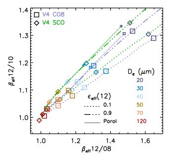
**Figure 10.** V4 ice LUTs, showing  $\beta_{eff} 12/08$  (*x* axis) vs.  $\beta_{eff} 12/10$  (*y* axis) for the CO8 model (squares and purple lines) and the SCO model (diamonds and green lines) for six values of  $D_e$  between 20 and 120 µm. The LUT values are shown for  $\varepsilon_{eff,12} = 0.1$  (dotted lines) and = 0.9 (dashed–dotted lines). The solid lines represent the approximate LUT values derived from Parol et al. (1991).
