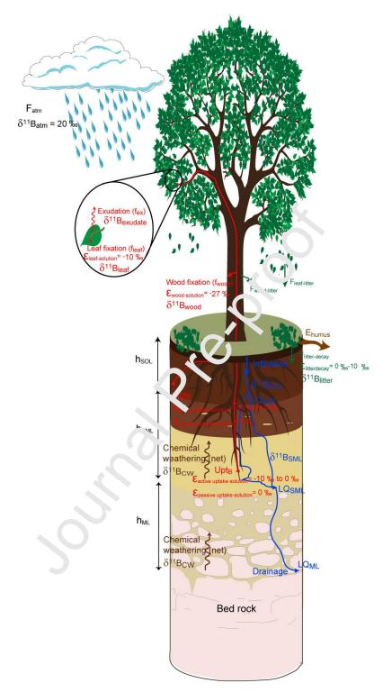
Figure 2: Evolution of the B isotopic composition of the soil solution in 3 different soil layers with the development of a forest for different supply rates of boron (atmospheric inputs,  $F_{atm}$  and chemical weathering, CW) and different B fractionation factors associated ( $\epsilon$ ) to the active uptake of boron by roots
