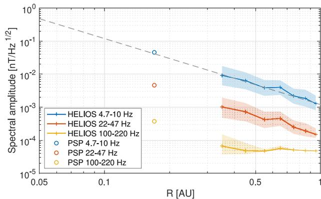
**Figure 2.** Average spectral amplitude of solar wind turbulence measured by the HELIOS search-coil at various distances from the Sun and by the SCM during the Venus encounter (at 0.5 AU). The dashed area for HELIOS refers to the 25%–75% quantile range. The dashed line represents the expected  $1/R^2$  scaling.
