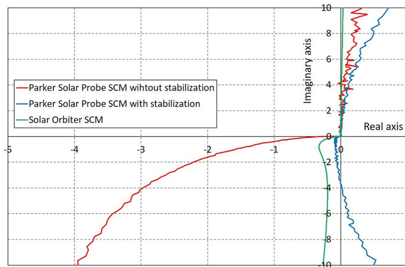
**Figure 6.** Nyquist plots of SCM open loop transfer functions for the Solar Orbiter (green) and Parker Solar Probe (red) instruments. The loop was open between the first amplification stage and  $R_{fb}$ . In this plot the abscissa axis represents the real part of the transfer function and the ordinate axis the imaginary part.
