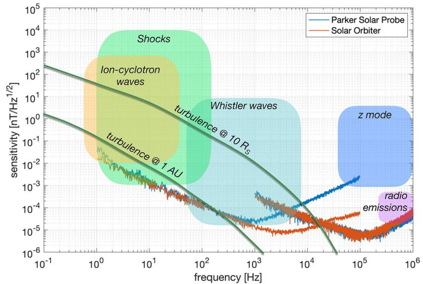
**Figure 1.** Sensitivity of the SCM sensors for Parker Solar Probe and Solar Orbiter with respect to the expected levels of magnetic fluctuations in the inner heliosphere (for one component of the magnetic field). The levels of turbulence at  $10 R_S$  are extrapolated from HELIOS observations made at 0.3 AU.
