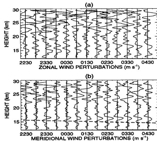
**Figure 2.** RD lidar profiles from 2230 LT on 23 October to 0500 LT on 24 October, 1995. The zero point of each profile is labeled with the starting time of its 30 min observational integration. Successive profiles are offset by  $10 \text{m s}^{-1}$ .
