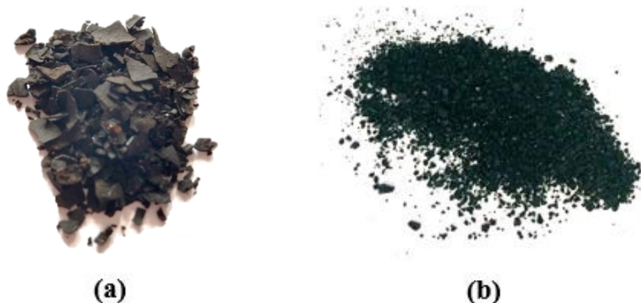
Figure 15. E. grandis lignin appearance: (a) before and (b) after the first desorption
