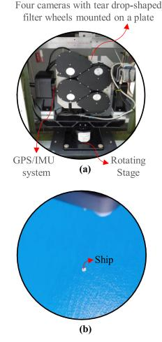
Fig. 2. (a) The NRL VICO instrument. (b) VICO true color image over the area of interest.
