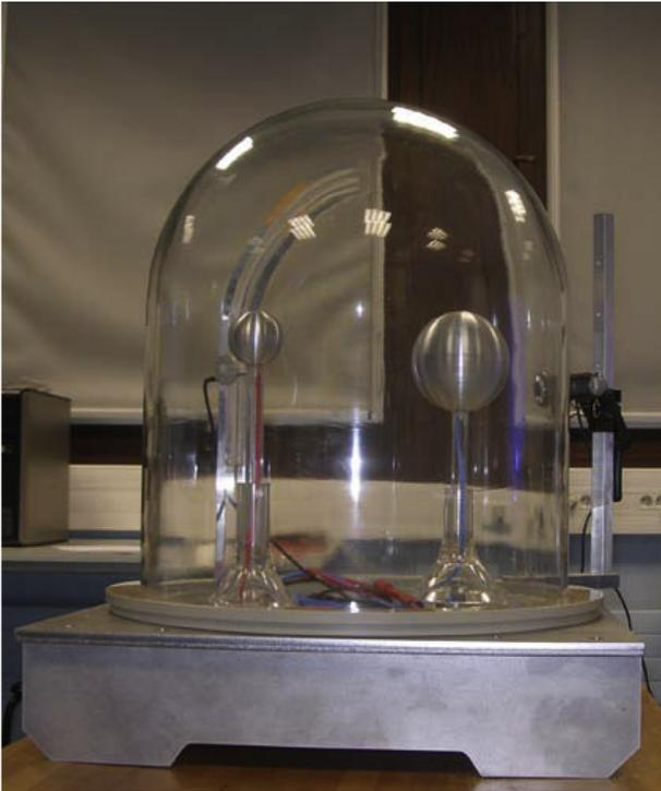
**Fig. 4.** *View of the Planeterrella II.* The vacuum chamber is in glass. The supports of the spheres are made such that they can move. For this purpose, the plate supporting the experiment had to be raised. On the right side, a small camera is hooked on a simple support. This support can rotate around the vacuum chamber. The external diameter of the vacuum chamber is 415 mm.
