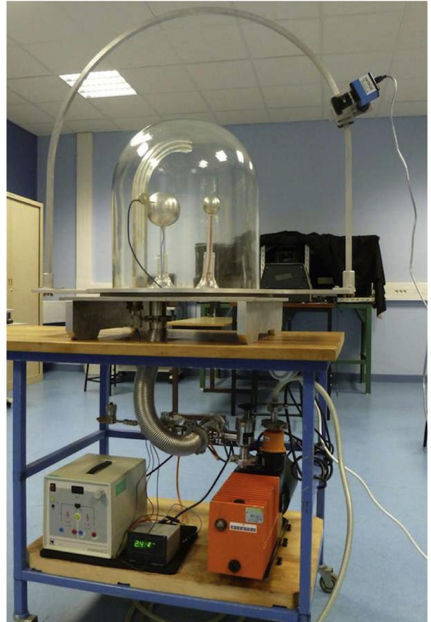
**Fig. 5.** *View of the Planeterrella III.* The camera is now hooked on an inverted-U support. The support can rotate around the vacuum chamber and the camera can move freely on this support. The supports of the spheres have been improved to allow now the spheres to rotate and not only to move forward. Here, the pressure is  $2.4 \times 10^{-2}$  mb.
