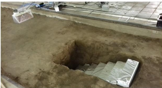
Figure 13: Illustration of the TUD experimental set-up for the “metallic staircase” experiment
