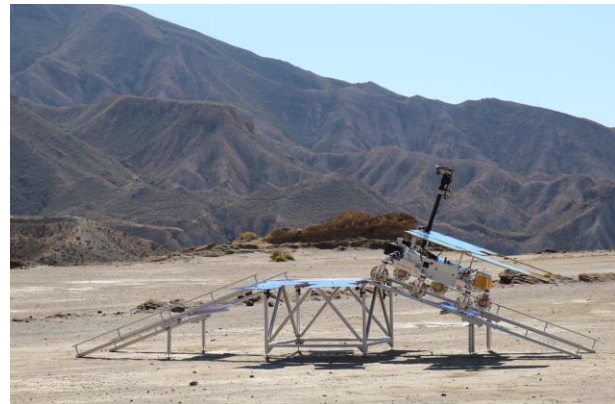
Fig. 1. Charlie on its way onto the landing platform in the Tabernas (Spain). PanCam is mounted on the mast, the drill box also containing CLUPI visible at the front and WISDOM at the back of the rover.
