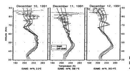
Figure 2. Comparison between ISAMS profiles and lidar profiles (Observatoire de Haute Provence, 44°N, 6°E).
