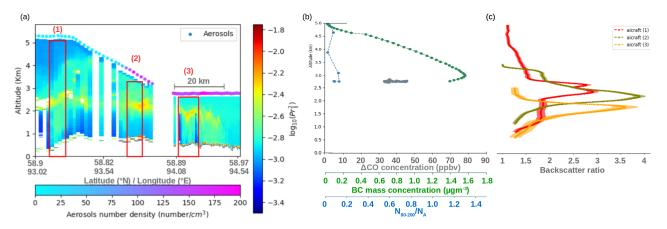
**Figure 11.** (a) Vertical cross-section of aircraft  $\log_{10}(PR^2)$  on 19 July 2013 at 06 UT. Calibration constant is 491,724  $\pm$  10%. Grimm aerosol concentrations in particle.cm<sup>-3</sup> are shown at the aircraft altitude. (b) Vertical profiles of  $\Delta$ CO in ppbv (grey), BC in  $\mu$ g.m<sup>-3</sup> (green) and ratio N<sub>80-200</sub>/N<sub>A</sub> (blue dashed line) for the descent at 94° E. (c) Backscatter ratio vertical profile for the lidar data in the red box.
