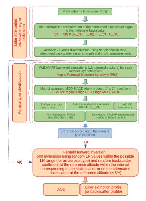
Figure 2. Flow chart of airborne lidar data processing and aerosol types identification.
