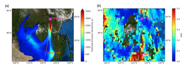
**Figure 23.** (a) as Figure 4a for the aerosol layer of Figure 22. Orange dotted line is the position of CALIOP overpass on 18 July 2013 at 18 U. (b) as Figure 4b with averaging of MODIS AOD<sub>550</sub> from 16 to 19 July 2013.
