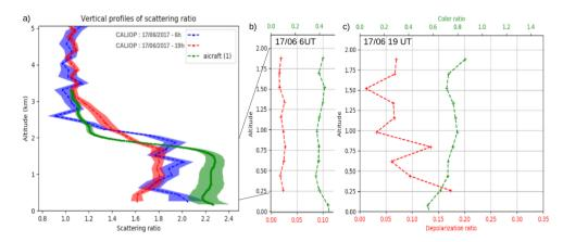
**Figure 17.** (a) Vertical profiles of 532 nm backscatter ratio for the aircraft lidar in red box of Figure 14a (red line) and for CALIOP on 7 June 2017 at, respectively 6 UT (56.7° N,83.7° E) and 19 UT (57.3° N, 87° E). (b) Vertical profiles of the particle color ratio (green) and particle linear depolarization ratio (red) measured by CALIOP on 7 June 2017 at 6 UT. (c) Vertical profiles of the particle color ratio (green) and particle linear depolarization ratio (green) and green and green
