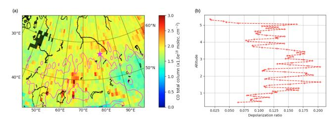
**Figure 5.** (a) Average of IASI tropospheric CO total column (in  $1.0 \times 10^{18}$  molecule.cm<sup>-2</sup>) from 13 to 16 June 2017. Pink isolines define areas with 10 µm AOD > 0.08. The pink star is the aircraft position on 16 June 2017. (b) CALIOP 532 nm particle linear depolarization ratio vertical profile in the aerosol source region at 49.7° N, 70° E (see Figure 4a).
