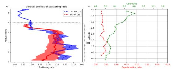
**Figure 10.** (a) Vertical profiles of 532 nm backscatter ratio for the aircraft lidar in red box of Figure 7a (red line) and for CALIOP on 18 June 2017 at 21 UT and 57° N (blue line). (b) Vertical profiles of the particle color ratio (green) and particle linear depolarization ratio (red) measured by CALIOP.
