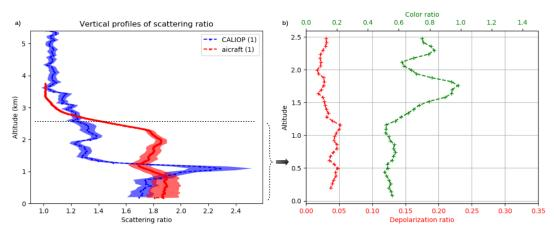
**Figure 6.** (a) Vertical profiles of 532 nm backscatter ratio for the aircraft lidar in red box of Figure 3a (red line) and for CALIOP on 15 June 2017 at 21 UT and 54° N, 75° E. (blue line), (b) Vertical profiles of the particle color ratio (green) and particle linear depolarization ratio (red) measured by CALIOP.
