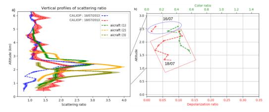
**Figure 13.** (a) Vertical profiles of 532 nm backscatter ratio for the aircraft lidar in red box of Figure 11a (red line) and for CALIOP on 16 and 18 July 2013 at, respectively 19 UT, 62° N and 05 UT, 59° N. (b) Vertical profiles of the particle color ratio (green) and particle linear depolarization ratio (red) measured by CALIOP.
