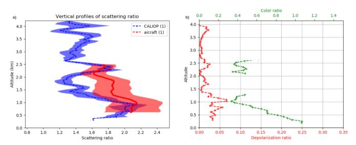
**Figure 21.** (a) Vertical profiles of 532 nm backscatter ratio for the aircraft lidar in red box of Figure 18a (red line) and for CALIOP on 17 July 2013 at 20 UT and 55.5° N (blue line), (b) Vertical profiles of the particle color ratio (green) and particle linear depolarization ratio (red) measured by CALIOP.
