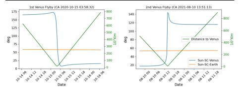
**Fig. 16** First and second Venus flybys linear and angular distances of the spacecraft: to the planet (green), to Sun and Venus (blue), to Sun and Earth (orange)
