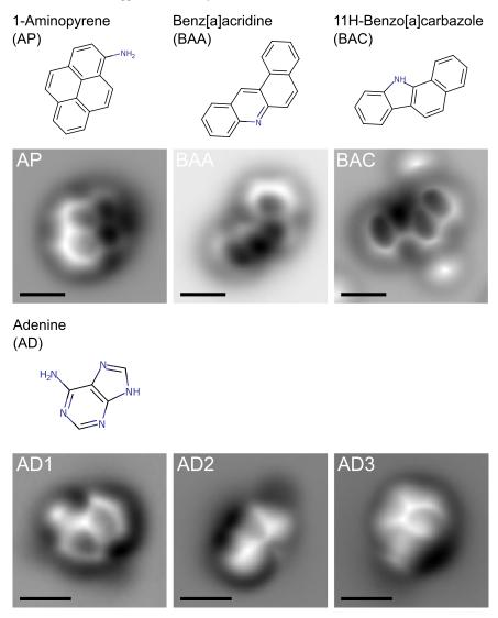
Figure A2. Molecular structure models and AFM images of nitrogen-containing model compounds. Images of AP, BAA, and BAC are acquired on NaCl(2ML)/Cu (111). Image AD1 is acquired on Cu(111) and AD2, AD3 on NaCl(2ML)/Cu(111). The two bright features adjacent to the molecule in the image of BAC are two CO molecules adsorbed on the NaCl film. All scale bars are 5 Ångström.
