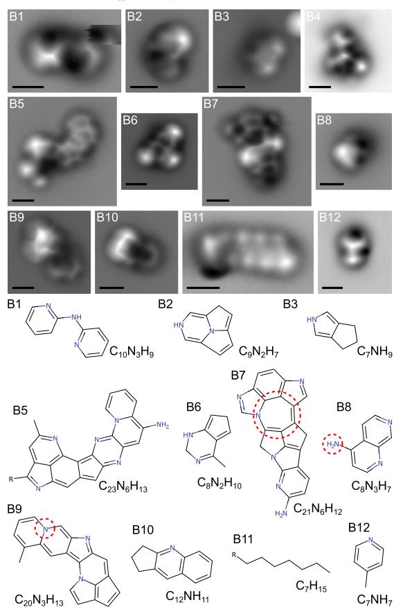
Figure 2. High-resolution AFM images and assigned structures of tholins from the insoluble fraction. All scale bars are 5 Ångström. Red dashed circles indicate uncertain moieties. A possible alternative assignment for the uncertain  $-NH_2$  group in B8 is a -CN group. Additional data obtained on the same molecules is presented in the Figures A4 and A5 in the Appendix.
