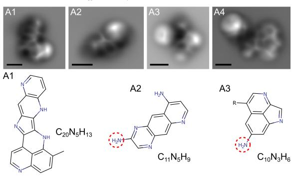
Figure 1. High-resolution AFM images and assigned structures of tholins from the common fraction. All scale bars are 5 Ångström. Red dashed circles indicate uncertain moieties. A possible alternative assignment for the uncertain  $-NH_2$  group in A2, A3 is a -CN group. Additional data obtained on the same molecules is presented in Figure A4 in the Appendix.
