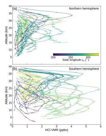
**Fig. 3.** Retrieved vertical profiles of HCl during the Mars year 35 dust season. The mean retrieved HCl VMR vertical profiles for each occultation made in a: the northern hemisphere, and b: the southern hemisphere during Mars year 35. Colours indicate solar longitude,  $L_s$ .
