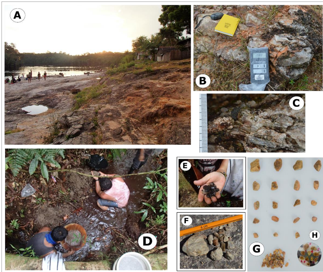
359 360 Figure 4. Pictures of field and mineral found in panning concentrates from LOC (5) San 361 Jose. A. view of rocks of Mitú complex in the Guainía River at San Jose indigenous 362 community; B. Pegmatite with an elevated radioactivity measures; C. Pegmatite with Fe- 363 columbite crystal; D. Sample site of heavy mineral concentration E. Fe-columbite crystals 364 from pan concentrates; F; Huge monazite crystals from pan concentrates; G. Monazite 365 crystals selected from the pan concentrates and H. Polished epoxy resin puck of monazite 366 for analysis.
