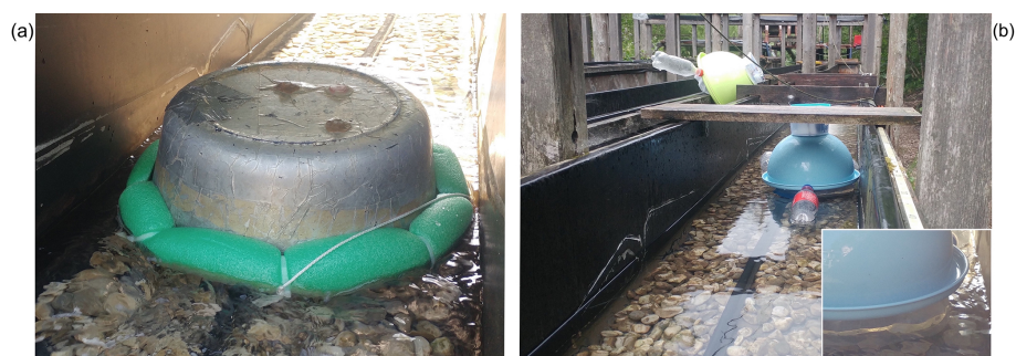
Figure 1. Two chamber designs: on (a) the standard chamber from Bastviken et al. (2015) and on (b) the flexible foil chamber (with a close-up of the peculiarity of the sealing).
