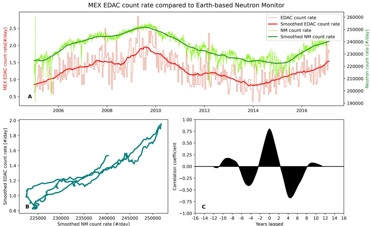
**Fig. 2.** Demonstration of the similar properties of the space-borne EDAC counter and the ground-based NM. *Panel A:* time series of the MEX EDAC count rate (red) and the McMurdo NM count rate (green). *Panel B:* smoothed EDAC rate as a function of the smoothed NM count rate. *Panel C:* cross-correlation between the two count rates; maximum correlation was found at exactly 0 lag, with a coefficient of 0.8.
