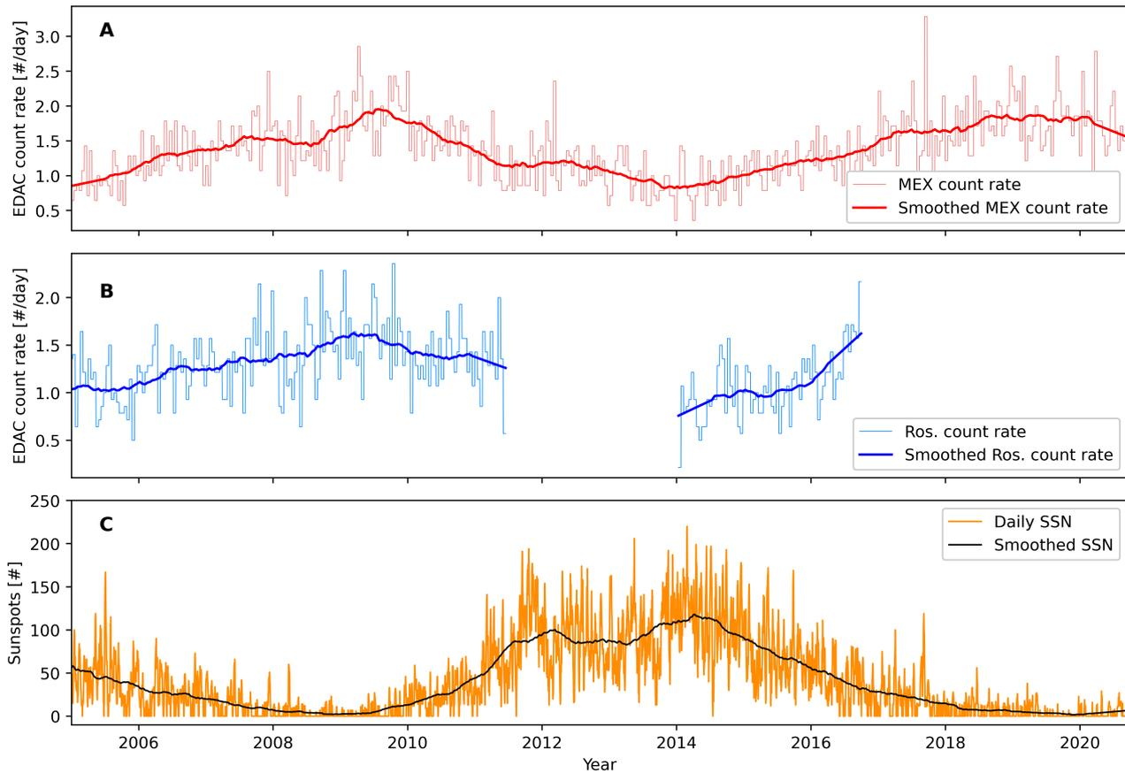
**Fig. 3.** Comparison between the two EDACs and the relevant solar cycle. *Panel A:* MEX EDAC daily count rates based on 14-day averages, with smoothed count rates. *Panel B:* Rosetta EDAC daily count rates based on 14-day averages, with smoothed count rates. *Panel C:* daily SSNs along with smoothed SSNs.
