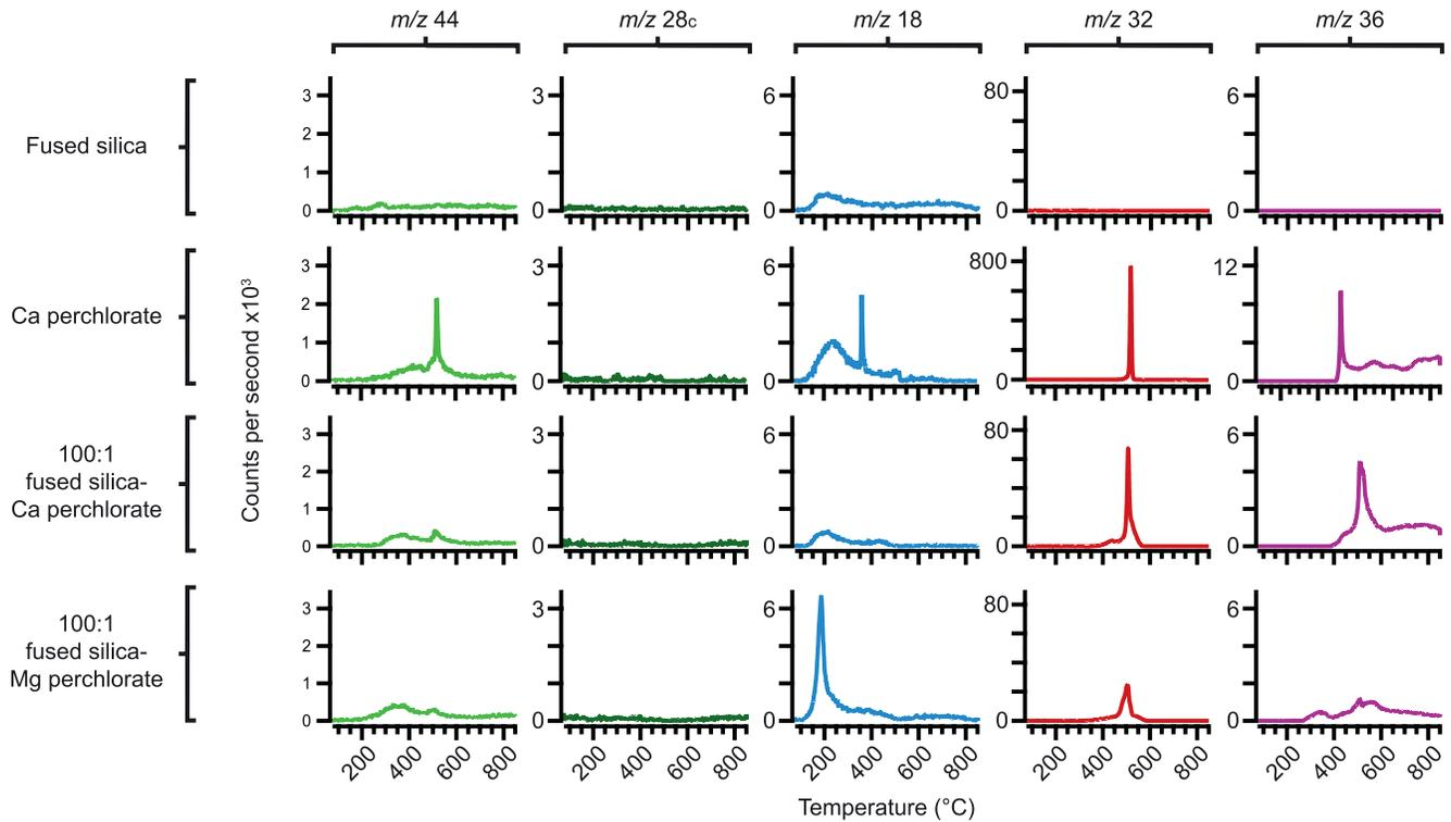
**Figure 1.** Evolved  $m/z$  44 ( $\text{CO}_2$ ),  $m/z$  28<sub>c</sub> (corrected CO),  $m/z$  18 ( $\text{H}_2\text{O}$ ),  $m/z$  32 ( $\text{O}_2$ ), and  $m/z$  36 ( $\text{HCl}$ ) versus temperature as detected by SAM-like EGA of the FS-120 fused silica, Ca perchlorate, a 100:1 fused-silica-Ca-perchlorate mixture, and a 100:1 fused-silica-Mg-perchlorate mixture. EGA, evolved gas analysis; SAM, Sample Analysis at Mars.
