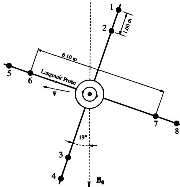
**Figure 5.** Schematic diagram (not to scale) of the TOPAZ III interferometer configuration and orientation at flight time 472.4 s. The perspective is from fore to aft along the spin axis of the payload and the payload spins counterclockwise. The antenna lie in the plane containing the magnetic field  $B_0$ , and payload velocity  $v$  (cartwheel attitude) which allows simultaneous measurements of parallel and perpendicular electric fields.
