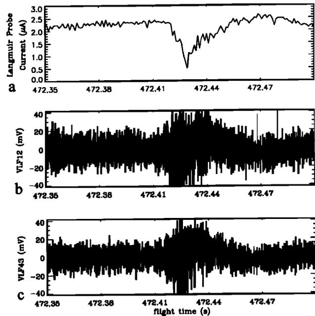
**Figure 6.** The time signature of the LHSS observed at 472.4 s flight time. (a) The fixed biased (+5 V) Langmuir probe current shows a 75% drop in measured current at this time indicating a deep density depletion. The LHSS structure is characterized by the sudden increase (472.41 s) and then decrease (472.45 s) in activity measured by the (b) VLF12 and (c) VLF43 channels.
