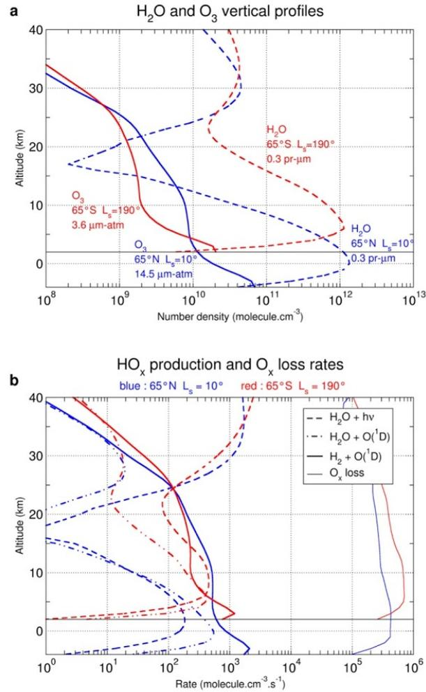
**Figure 4.** Examples of profiles of O<sub>3</sub>, H<sub>2</sub>O, and production/loss rates calculated by the LMD GCM at high latitudes in early spring. Altitude is relative to the Mars areoid and local time is 1200. (a) O<sub>3</sub> and H<sub>2</sub>O number densities at 65°N (L<sub>s</sub> = 10°) and 65°S (L<sub>s</sub> = 190°). (b) HO<sub>x</sub> production rate for the most important reactions and O<sub>x</sub> loss rate at 65°N (L<sub>s</sub> = 10°) and 65°S (L<sub>s</sub> = 190°).
