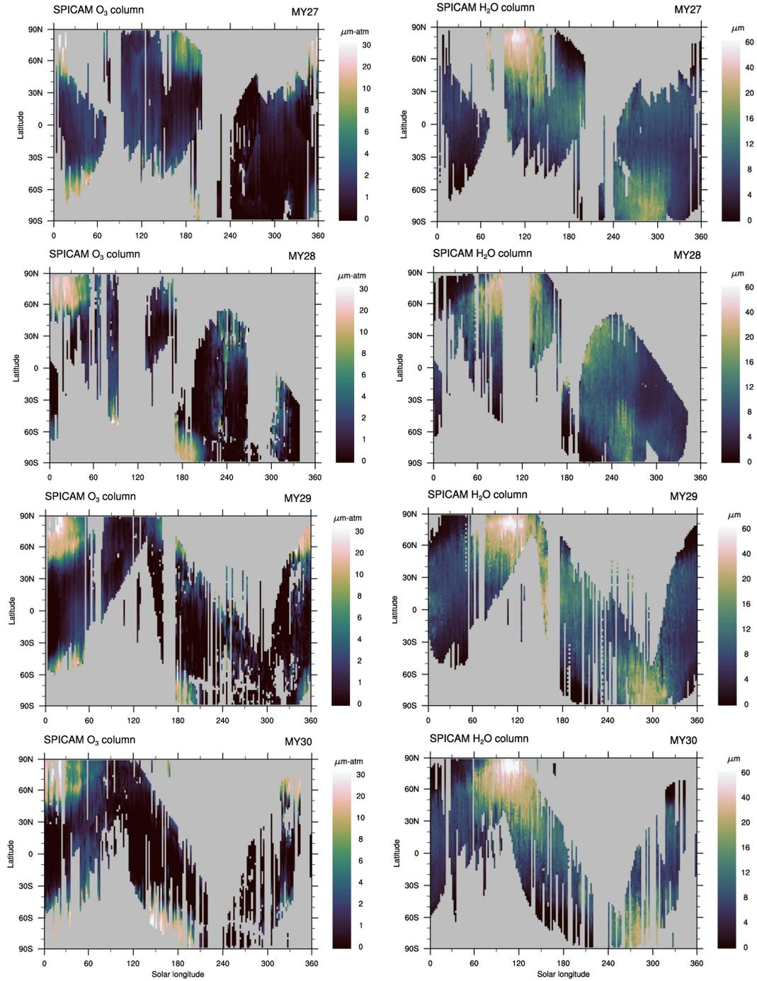
**Figure 1.** Overview of the SPICAM ozone (left) and water vapor (right) column abundance as a function of season, latitude, and Mars year. The columns are zonally averaged and binned by  $2^\circ$  in  $L_s$  and  $2^\circ$  in latitude. Units are micron-atmosphere ( $\mu\text{m-atm}$ ) for ozone and precipitable micron ( $\text{pr-}\mu\text{m}$ ) for water vapor.
