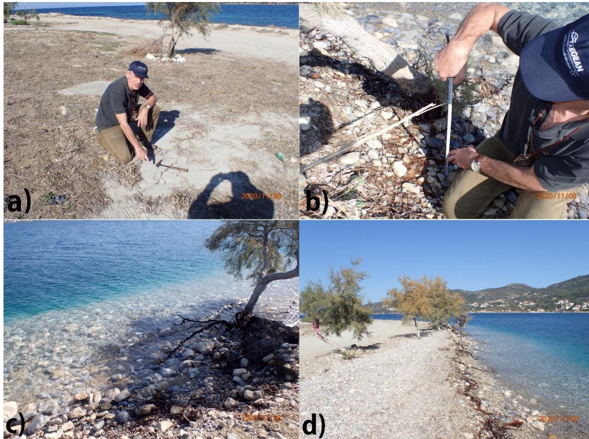
Fig. 10. Field photographs showing earthquake-induced failures at Malagari, Samos (see Fig. 9 for its location, opposite to the town of Vathy) a) liquefaction b) coastal subsidence of 53 cm c) submergence of former beach d) submerged tree line.
