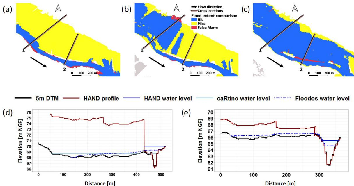
**Figure 7.** Simulation results on the Argent-Double river at La Redorte, showing large differences between the three tested approaches, including (a) HAND/MS, (b) caRtino 1D, and (c) Floodos. (d) Cross section 1, comparing water surface and terrain elevations and the HAND profile (addition of the HAND height values and the elevation of the drainage point in the section), and (e) cross section 2 (same information as cross section 1).
