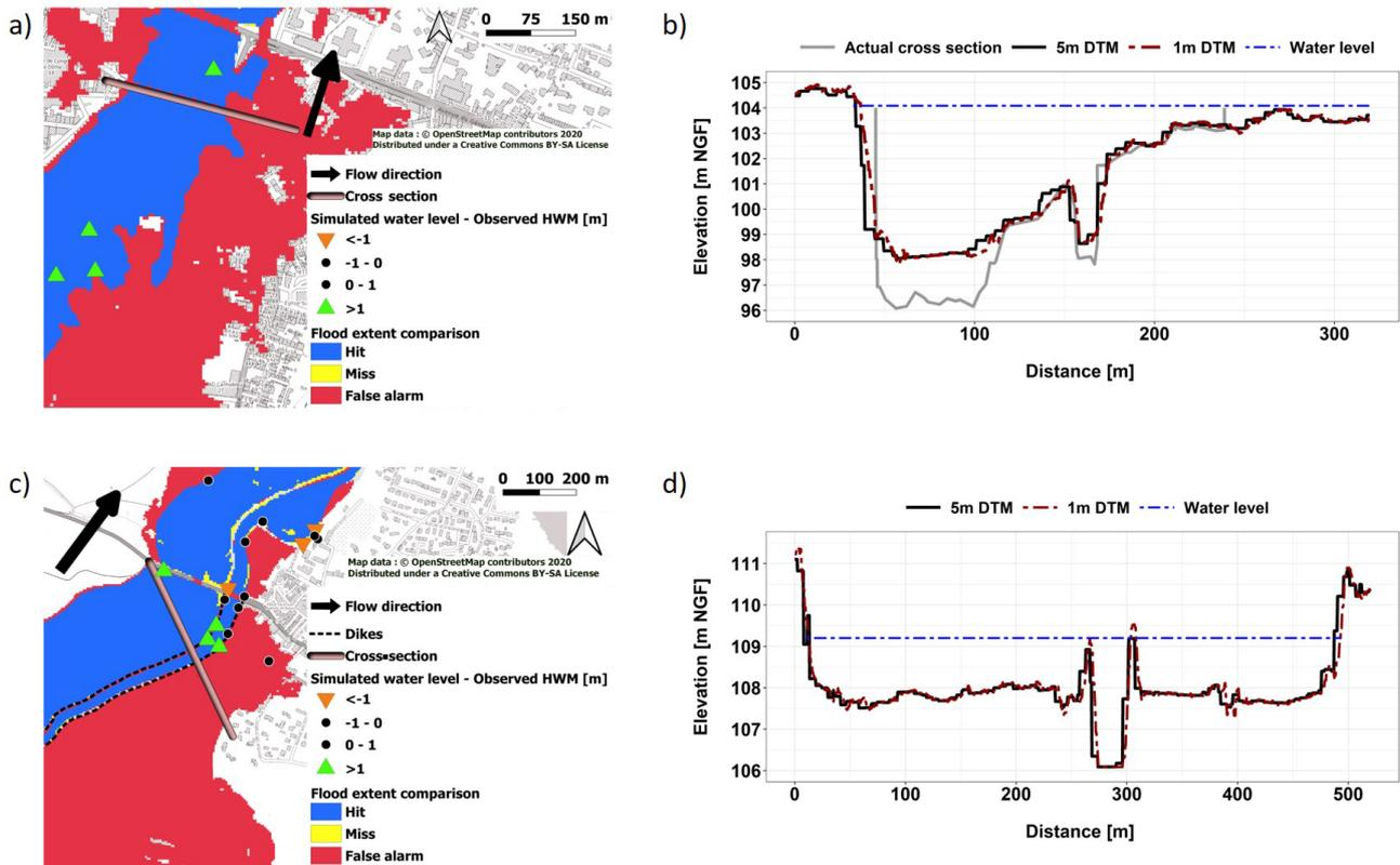
**Figure 8.** Illustration of errors induced by the limitations of the DTM. (a) Aude river at Carcassonne – simulation results (Floodos model). (b) Aude river at Carcassonne – cross sections and simulated water level. (c) Fresquel river at Pezens – simulation results (Floodos model). (d) Fresquel river at Pezens – cross sections and simulated water level.
