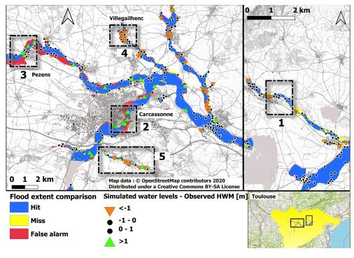
Figure 4. Simulated and observed flood areas and water levels for the Aude 2018 event and the Floodos simulation approach.
