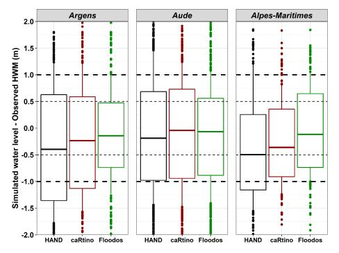
**Figure 6.** Comparison of simulated water levels and observed high water marks (HWMs) for the three methods and the three events. The box plots represent, respectively, the 5 % and 95 % (whiskers) and the 15 % and 85 % quantiles (boxes).
