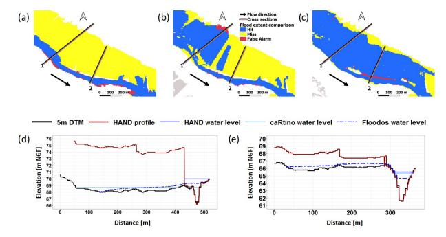
**Figure 7.** Simulation results on the Argent-Double river at La Redorte, showing large differences between the three tested approaches, including (a) HAND/MS, (b) caRtino 1D, and (c) Floodos. (d) Cross section 1, comparing water surface and terrain elevations and the HAND profile (addition of the HAND height values and the elevation of the drainage point in the section), and (c) cross section 2 (same information as cross section 1).
