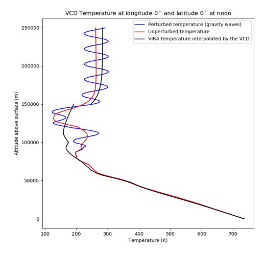
**Figure 4:** Illustrative example of a climatological temperature profile, along with a perturbed one (using the small-scale perturbation scheme) and VIRA reference values.
