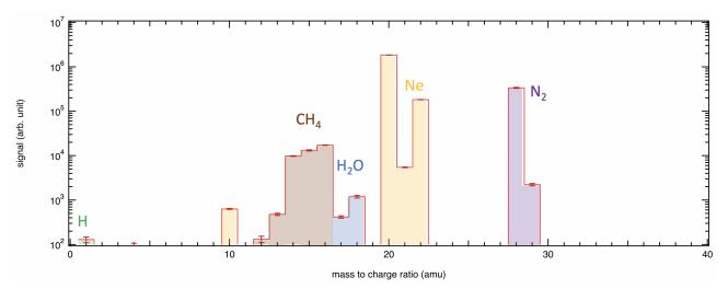
Fig. 1. In situ non-normalized gas-phase m/z spectrum of neutral species present in the reactor before EUV irradiation.
