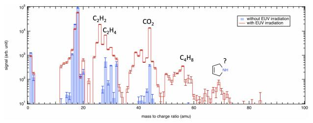
Fig. 2. Ex situ experimental m/z spectra obtained for neutral species with a N<sub>2</sub>-CH<sub>4</sub>-H<sub>2</sub>O gas mixture with (red) and without (blue) irradiation in the photochemical chamber by using a 3-hour cryogenic trapping system.
