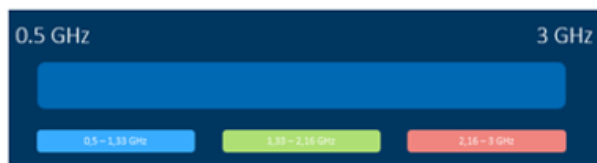
Figure 3 Illustration of the whole frequency bandwidth split into 3 frequency sub-bands,
