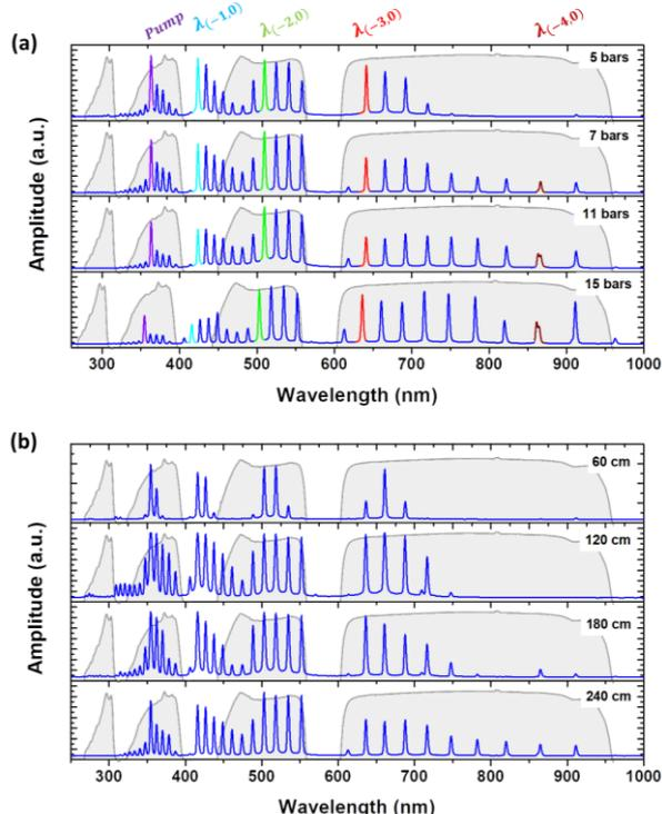
Fig. 2. (a) Comb spectra obtained by using  $\text{H}_2$  at 5, 7, 11, and 15 bar for a 180 cm fiber length. (b) Comb spectra for fibers with lengths of 60, 120, 180, and 240 cm filled with  $\text{H}_2$  at 5 bar.
