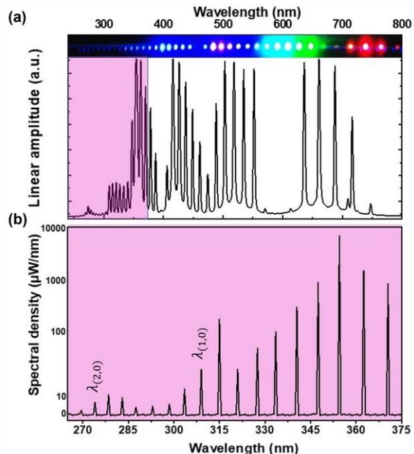
Fig. 3. (a) Comb spectrum for a fiber with length 120 cm and filled with  $\text{H}_2$  at 5 bar. The diffracted output comb pattern is displayed on the figure top part. (b) Zoom in the wavelength range between 265 nm to 375 nm.
