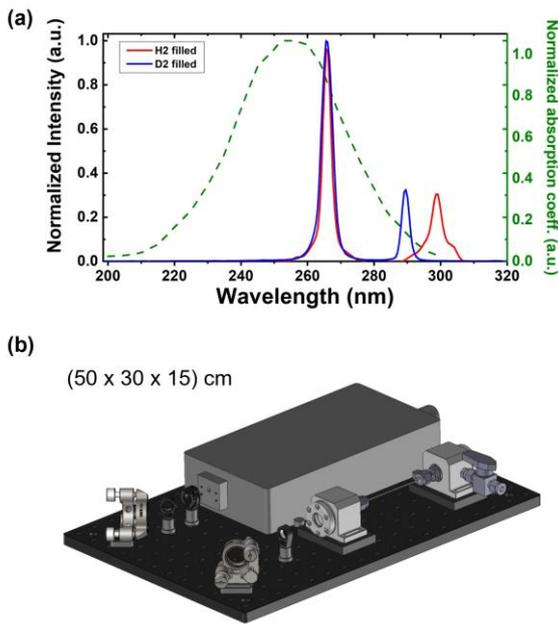
Fig. 4. (a) Raman generation plots in a 25 cm D<sub>2</sub>-filled fiber (blue curve) and in a 7 cm H<sub>2</sub>-filled fiber (red curve). The green curve represents the normalized absorption coefficient of ozone in the Hartley band. (b) Diagram of the HCPCF-based DIAL LIDAR source reported herein with its typical dimensions.
