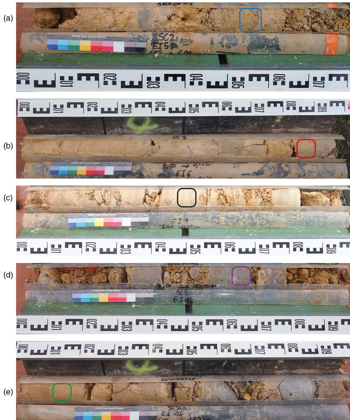
FIGURE 7 Core samples of the interval: (a) 4.6–6.0 m, (b) 6.0–7.0 m, (c) 7.0–8.0 m, (d) 14.0–15.0 m, and (e) 16.0–17.0 m for B2. The rectangles represent the R_A sample in blue, the R_B sample in red, the R_C sample in black, the R_D sample in purple, and the R_E sample in green
