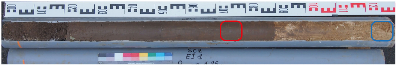
FIGURE 4 Core samples of the interval 0.0–1.3 m for B2. The rectangles represent the S_B sample in red and the P_A sample in blue
