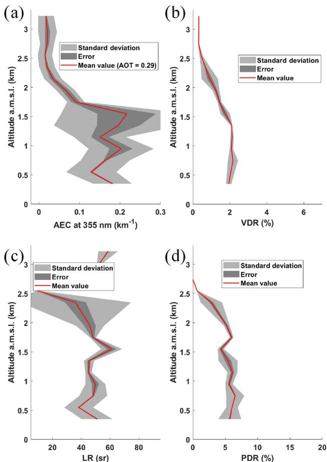
**Figure 5.** Vertical profiles derived from ALiAS during flight 07 on 31 January 2020 at 15:00–18:45 UTC of (a) the aerosol extinction coefficient (AEC), (b) the volume depolarization ratio (VDR), (c) the lidar ratio (LR), and (d) the particle depolarization ratio (PDR).
