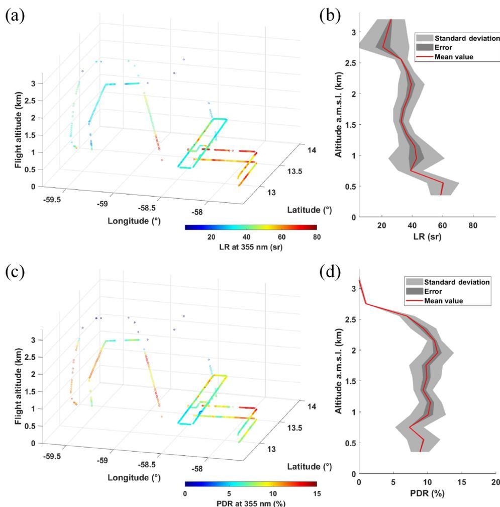
**Figure 6.** (a) Lidar ratio (LR) derived from ALiAS measurements during the flight F10 on 2 February 2020 at 19:45–21:00 UTC; (b) corresponding vertical profile of the LR which shows the spread of measurements via the standard deviation (light-grey area) and the statistical error (dark-grey area). The same types of figures are given for the particle depolarization ratio (PDR) in panels (c) and (d), respectively.
