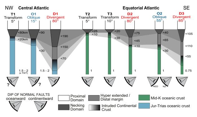
**Figure 8.** Summary of the main crustal structure characteristics of the Guiana shield margin segments. Values are dip width of the crustal domains in km except for the oceanic crust for which the thickness in TWT in seconds is indicated. See location of segments on Figure 2.
