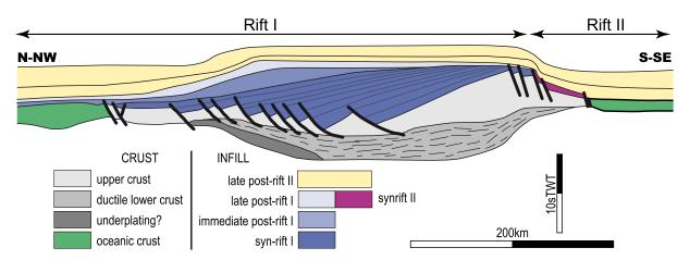
Figure 11. Schematic cross-section across the Demerara Plateau continental block illustrating the difference in necking style and thinning processes between the CAR (Rift I) and the EAR (Rift II).
