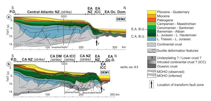
Figure 5. Geological cross sections through the northern edge of the Demerara Plateau across the (a) T2 and (b) T3 transform segments. See location on Figure 2. CA, Central Atlantic; EA, Equatorial Atlantic; HED, hyper extended domain; ICC, intruded continental crust; ND, necking domain.
