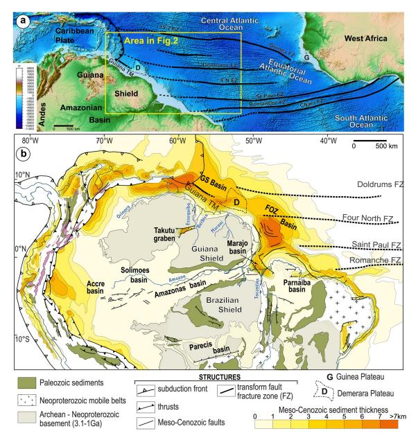
**Figure 1.** (a) Location of the study area. (b) Simplified geological map of northern South America showing the context of the Guiana Shield and its margin with Meso-Cenozoic sediments thickness (modified after Cordani et al., 2016). FOZ, Foz d'Amazonas; FZ, transform fracture zone; GS, Guiana-Suriname; TM, transform margin. Topography and bathymetry after NOAA (2009).
