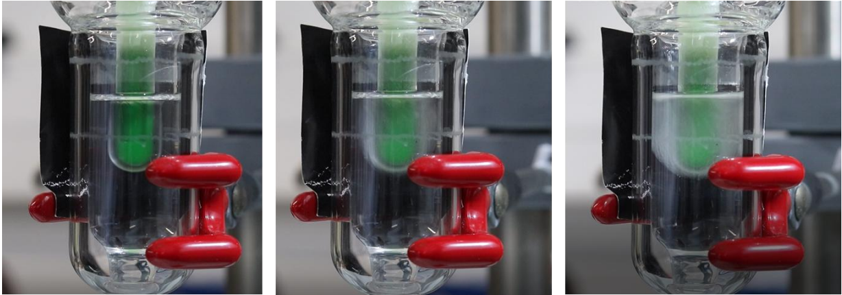
Figure S2: Examples of time-lapse photography, used to calculate speed and shape of freezing at 0 minutes, approximately 15 minutes and 40 minutes ( 35 \text{ g kg}^{-1} \text{ NaCl} )
