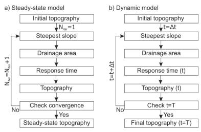
**Figure 1.** Overview of the algorithms used for the a) steady-state and b) dynamic simulations.
