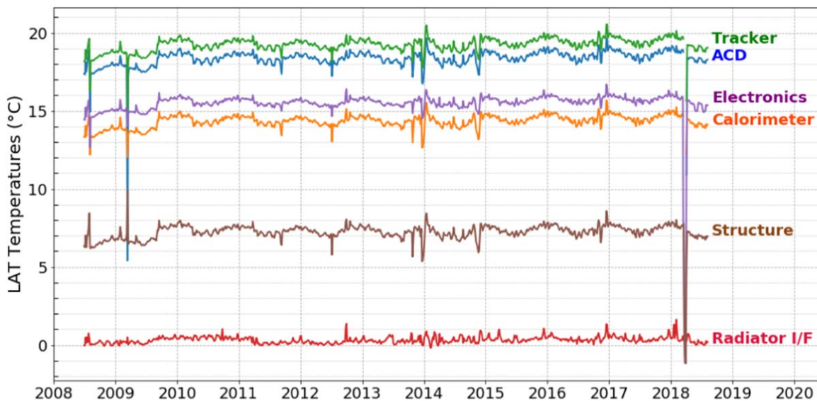
Figure 3. Temperatures ( ^{\circ}\text{C} ) of various parts of the LAT as a function of time, in years. Long-term temperatures are quite stable with small annual variations and excursions due to fixed orientations and other reasons, with the larger changes and recoveries in 2008, 2009, and 2018 due to LAT power outages.
