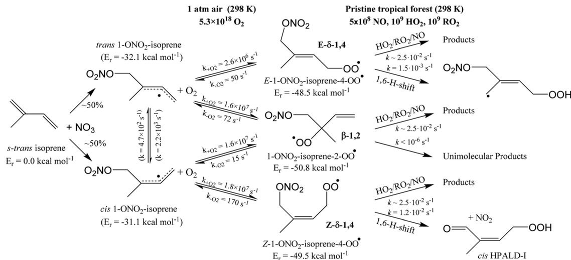
Fig. 2 Reaction scheme for the site-specific addition of  $\text{NO}_3$  on C1 of isoprene, and the subsequent stereo-specific addition of  $\text{O}_2$ . The ESI† includes schemes for  $\text{NO}_3$ -addition on carbons C2, C3 and C4. Co-reactant concentrations are taken as in Peeters *et al.*<sup>12</sup>
