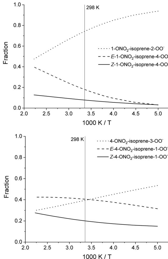
**Fig. 3** Temperature-dependent equilibrium population contribution for the individual RO<sub>2</sub> isomers formed after NO<sub>3</sub> addition to C1 (top) or C4 (bottom) of isoprene.
