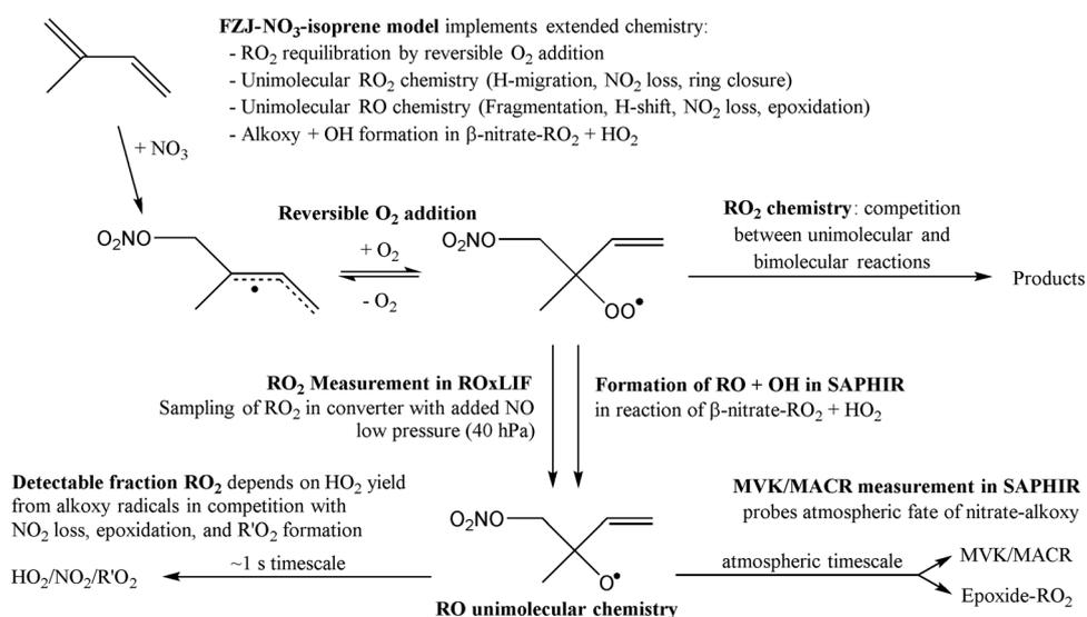
**Fig. 1** Summarizing scheme showing the investigated steps, which includes the NO<sub>3</sub> and (reversible) O<sub>2</sub> addition (site- and stereospecificity omitted), unimolecular chemistry of the nitrate peroxy and alkoxy radicals, and interpretation of the experimental RO<sub>2</sub> and MVK/MACR measurements. All chemistry is implemented in the FZJ-NO<sub>3</sub>-isoprene model.
