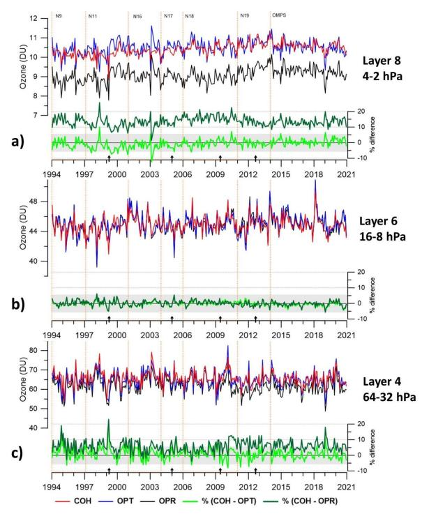
Figure 7. The time series of ozone at Boulder in Umkehr layer 8 (2-4 hPa). Operational Umkehr (black), Optimized Umkehr (blue) and COH (red) data are shown as monthly averages. Difference between COH and Operational Umkehr data is shown
