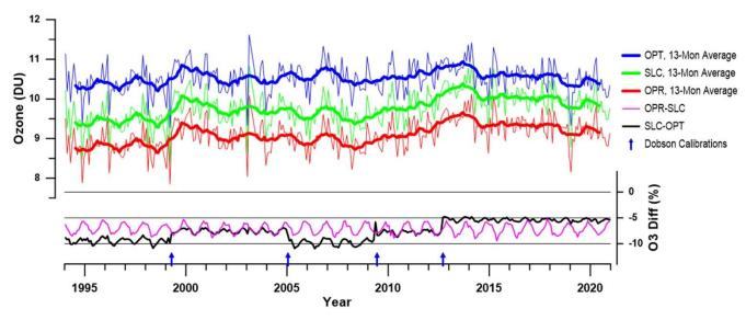
Figure 4. Upper panel: The time series of Umkehr monthly averaged (thin lines) ozone in layer 8 (4-2 hPa) compare operational (OPR), standard stray light corrected (SLC) and optimized (OPT) versions. The thick lines are 13-months running smoothing. Lower panel: a difference between OPT and SLC (black line), and between OPR and SLC data (purple line).
