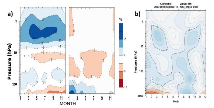
Figure 6. Seasonal biases between the Umkehr measurements in Boulder and the COH record from 2005 to 2018. Two panels show results for Umkehr retrievals: operational (left), Optimized correction (right). The biases are significantly reduced after the Optimized Umkehr correction. The right panel is the difference between Umkehr 11b (McPeter and Labow, 2011) and OMPS a priori (Flynn et al, 2014).
