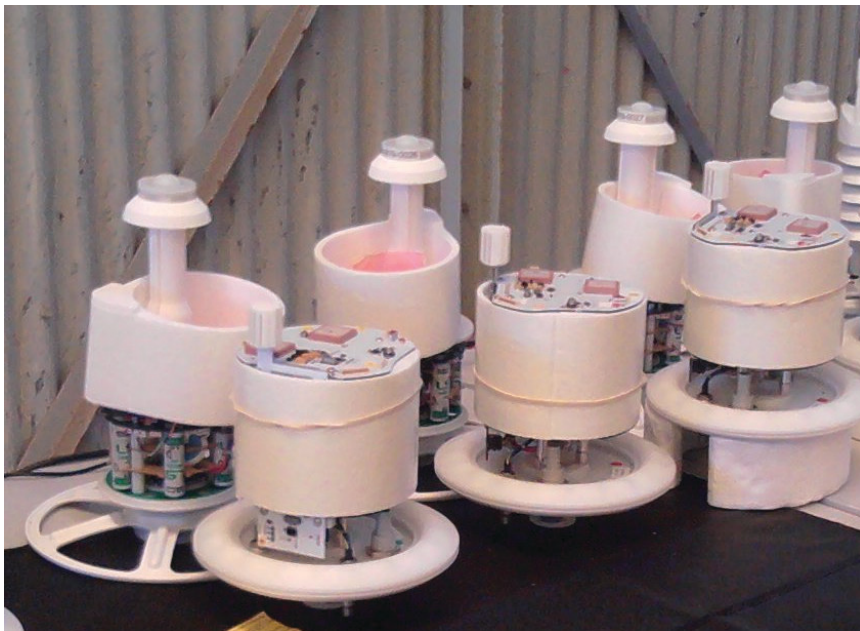
FIG. 4. Gondolas used during SAF-MED (2013) before being mounted on the balloons. SPH gondolas are in the front row. The cover of the base of the NPS is in a lifted position, so the batteries are visible, and the aspirated radiation shield that contains the temperature and humidity sensor is hidden. The global radiation sensor can be seen at the top of the NPS gondolas. (Photo credit: CNES.)
