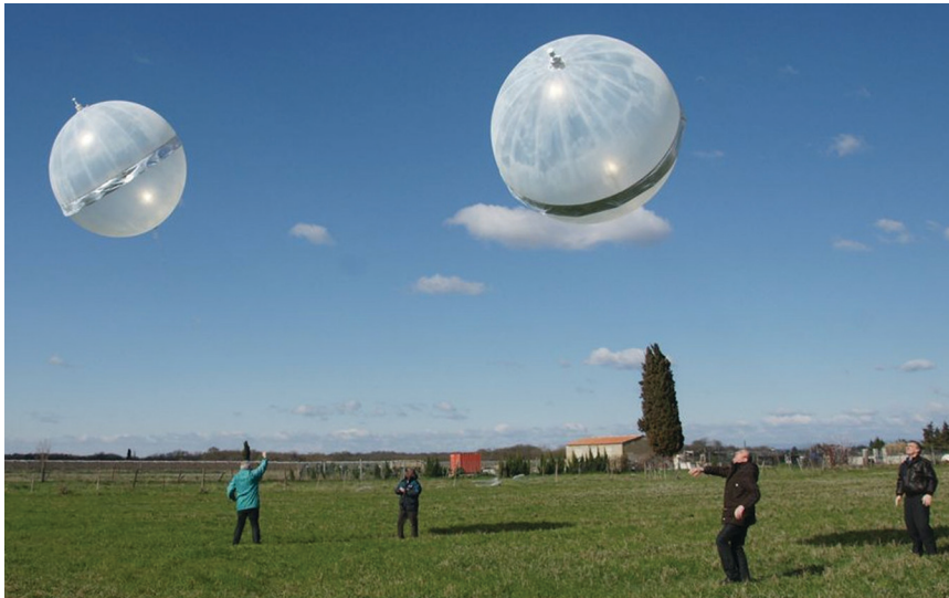
FIG. 1. Simultaneous launch of two BLPBs during the winter SOP of HyMeX, on 14 Mar 2013 in Candillargues (France). Note the external scientific gondola at the top of the balloon and the shiny belt that is the rain deflector, as well as the nontransparency of the balloons as they are coated with a rain repellent. (Photo credit: CNES.)
