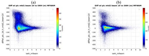
Figure 4 Histogram of the differences between SWIM and MFWAM peak wavelengths as a function of significant wave height. (a) when the SWIM peak wavelengths is estimated on the omni-directional wave height spectrum without any prior filtering (b) same but with filtering on the 2D wave slope spectra. The data set is from 2020-01-26 to 2020-02-06, processed with the version V5.0.
