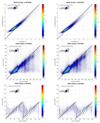
Figure 1 : histogram of wave parameters from CFOSAT-SWIM (beam 10 deg) vs MFWAM wave parameters ( 2019 April 26<sup>th</sup> -08<sup>th</sup> May), with the previous speckle noise correction (left), and the new speckle noise correction (right). Top: significant wave height; middle: peak wavelength; bottom: dominant direction.
