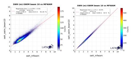
Figure 2 SWIM wave parameter SWH from 10°beam data compared to MFWAM SWH, for MTF1 (left and MTF3 (right). The period of observations is 26 January 2020 to 6 February 2020
