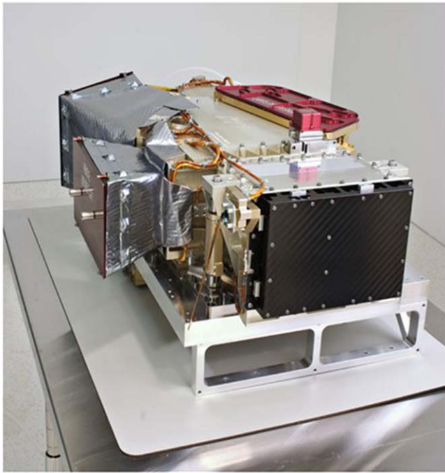
Figure 23. MAVEN IUVS instrument, described in McClintock et al. (2015). Covers over the two apertures are in place in this photograph, with one shown on the left of the image.
