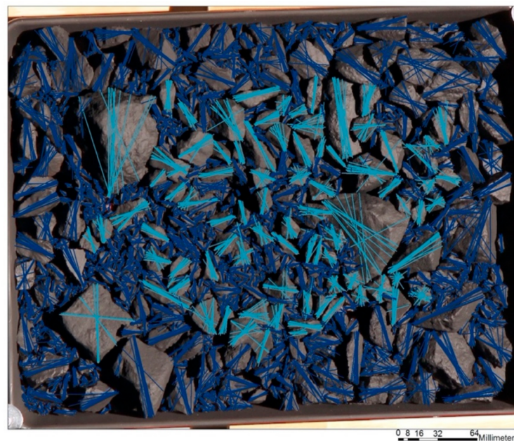
Figure 3. Rock Tray 1 from the OSIRIS-REx particle measurement uncertainty analysis with remotely measured counts overlaid. Counts were performed in the same ArcMap mapping environment used for mission operations. Counters who mapped in ArcMap mapped the full image, but ground-truth caliper measurements were only collected for 85 of these rocks (shown in light blue).
