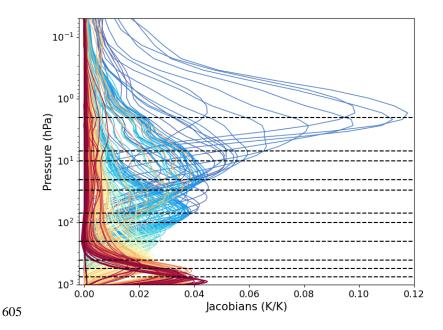
Figure 2: Jacobians for the 231 selected IASI channels. Horizontal dashed lines represent the 11 pressure levels for which the temperatures are computed. The colors of the jacobians represent the wavenumbers of the selected channels (blue for the channels around 700 cm<sup>-1</sup>, red for the channels around 2200 cm<sup>-1</sup>).
